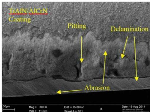
Figure 1 Several failure modes during machining of Inconel 718.
