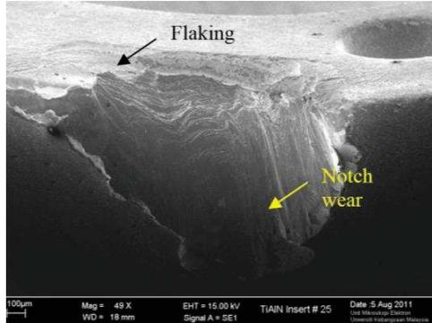
Figure 2 Failure mode observed during catastrophic failure.
