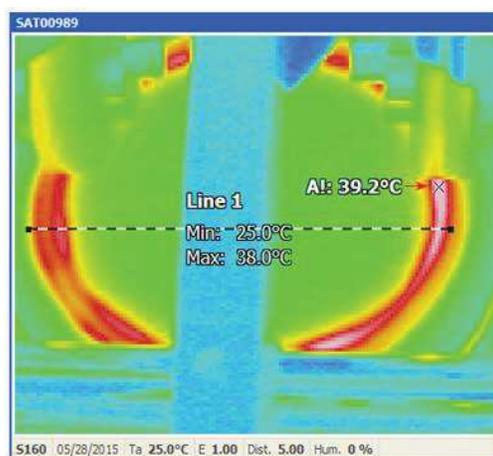
Figure 3 Thermal distribution at abrasion wheel.
