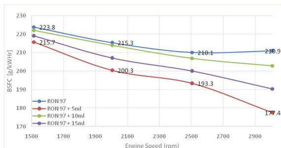
Figure 1 Engine speed Vs BSFC.
