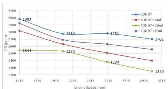
Figure 2 Graph of CO vs engine speed.
