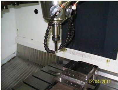
Figure 2 MQL experiment setup.
