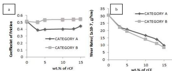
Figure 2 (a) Coefficient of friction and (b) wear rates of category-A and category-B composites.
