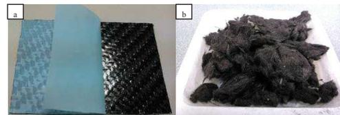
Figure 1 (a) Waste of carbon fiber prepreg (rCFP) and (b) crushed rCFP after cleaning with acetone for category-B composites.
