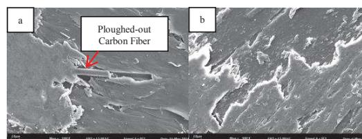
Figure 3 SEM micrographs of a (a) category-A composites for rCFP with resin and (b) category-B composites for rCFP without resin (x500).
