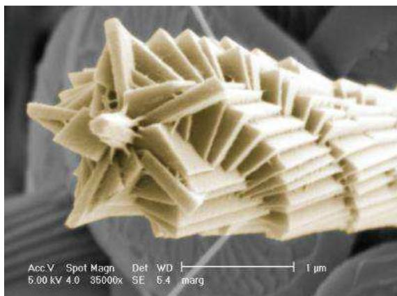
Figure 1 Spine tip of the microorganism *Rhabdosphaera clavigera*. Material: Calcite,  $\text{CaCO}_3$ . Structure: spiral formed from consistently aligned crystal units with rhombic faces. Process: Biomineralized in cool seawater, with the help of proteins, at ambient conditions. Scale bar  $1 \mu\text{m} = 0.001 \text{ mm}$ . [11]
