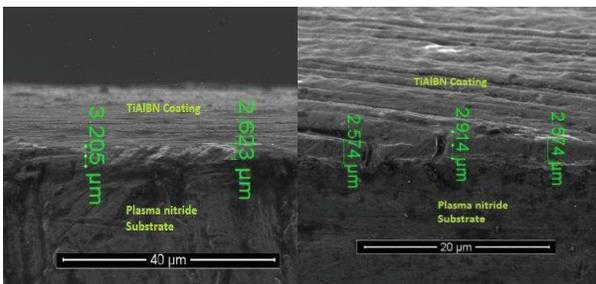
Figure 1 SEM micrograph of the (a) TiAlBN duplex sample with 1 hour plasma nitriding treatment (b) TiAlBN duplex sample with 3 hours plasma nitriding treatment.
