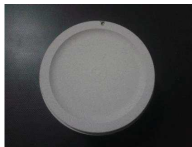
Figure 1 Actual plasma sprayed Mullite coated piston crown.
