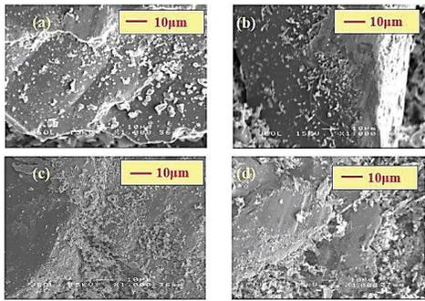
**Figure 2:** Numerous wear debris of the size below 10  $\mu\text{m}$  observed in tests with silicon carbide (a) and (b) but lesser wear debris with (c) silica sand and (d) garnet
