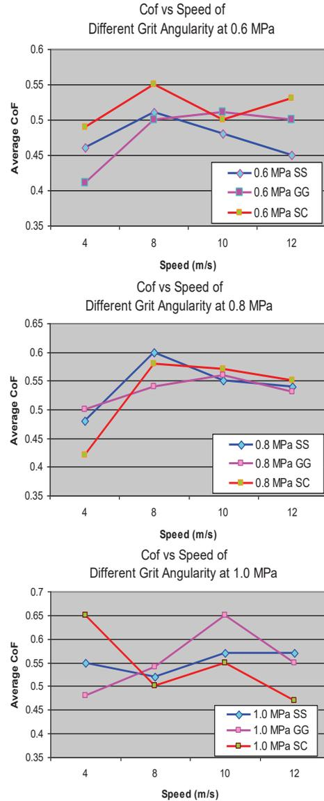
**Figure 3:** CoF values for the three grit particle types during drag mode and hard braking test
