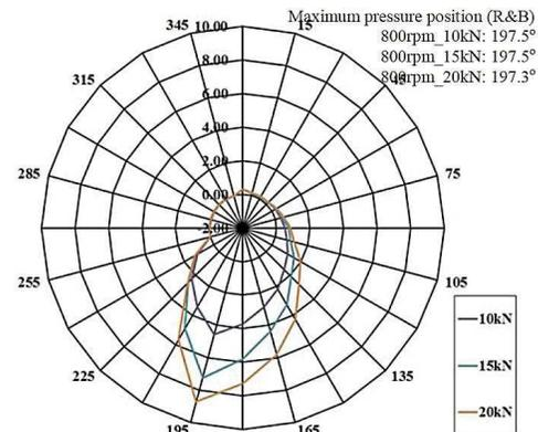
**Figure 6:** Oil pressure profiles of journal bearing at 800 rpm for speed of 10kN, 15kN and 20kN.
