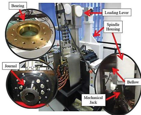
**Figure 4:** An assembly of journal bearing test rig.
