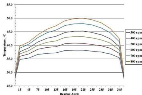
**Figure 5:** Oil temperature profiles in journal bearing at 10kN load for speeds of 300, 400, 500, 600, 700 and 800 rpm.
