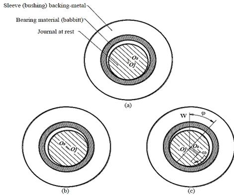
**Figure 2:** Schematic diagram of bearing positions at (a) start-up, (b) no load and (c) steady running conditions.
