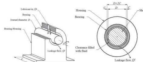
**Figure 1:** Journal bearing geometry and nomenclature (adapted from [1]).
