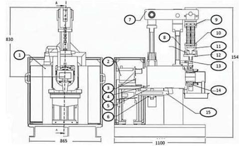
**Figure 3:** An assembly diagram of journal bearing test rig. 1) Frame, 2) Motor, 3) Motor bracket, 4) Spindle assembly, 5) Bellow top plate, 6) Bellow guide plate, 7) Loading Lever, 8) Pivot assembly, 9) Chain, 10) Chain holder, 11) Load Cell holder, 12) Load Cell, 13) Loading plate, 14) Bearing unit and 15) Pneumatic bellows.
