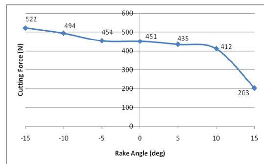
**Fig.6. Effect of increase of rake angle of DNMA to cutting force**
