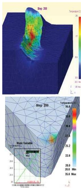
**Fig.12. Generated temperature on chip, work piece and tool edge when set up of rake angle +15**
