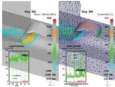
**Fig.5. Example of the simulation result for cutting speed at 200 m/min (300 steps)**
