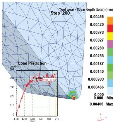
Fig.8. Wear depth for rake angle 0 maximum wear depth reached 0.00466 mm
