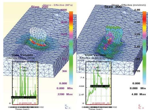
**Fig.14. Stress and strain on chip and material surface when set up of rake angle +15**
