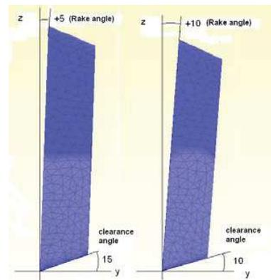
Fig.11. Change of the rake angle in 5 deg, cause the clearance changed conversely in 5 deg
