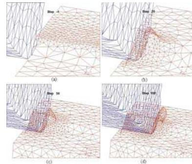
**Fig.4. (a) Initial mesh and tool indentation, (b) Chip formation at step 25, (c) Chip formation at step 50, (d) Developed continues chip at step 100.**
