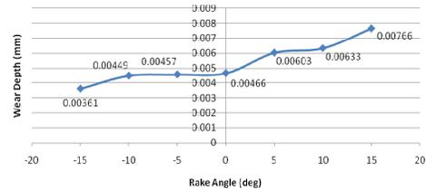
Fig.10 Effect of increase of rake angle of DNMA to wear depth (decreasing of clearance angle).
