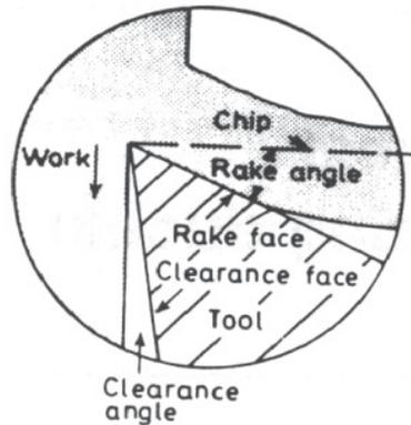
**Fig.1. Terminology of Cutting tool and Workpiece material**
