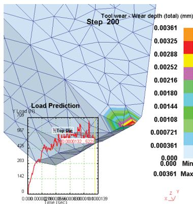
Fig.9. Wear depth for rake angle -15, the maximum wear depth reached 0.00361 mm
