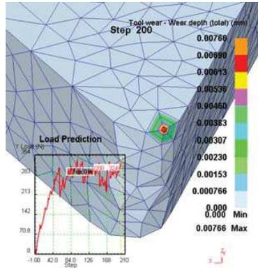
Fig.7. Wear depth for rake angle +15 maximum wear depth reached 0.00766 mm
