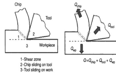
**Fig.13. Heat generated and heat dissipation in metal cutting [14]**
