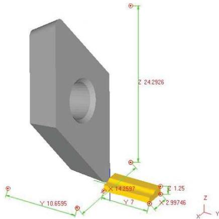
**Fig.2. Geometry and schematic of orthogonal cutting condition model**
