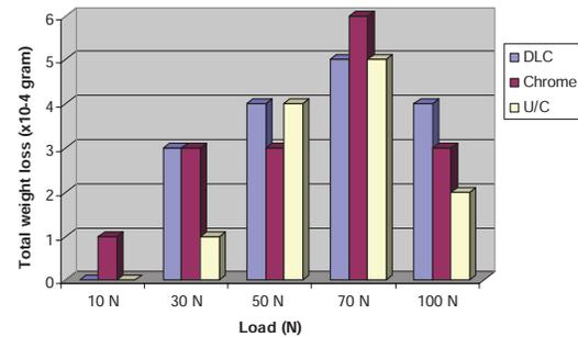
**Fig.8 Total weight loss for all specimens (pins and plates)**
