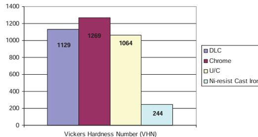
Fig. 2 Vickers Hardness Number for all material samples at 10kgf
