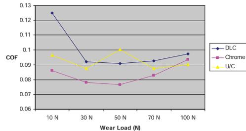
Fig.6 Coefficient of friction (COF) vs. load (N) for all samples
