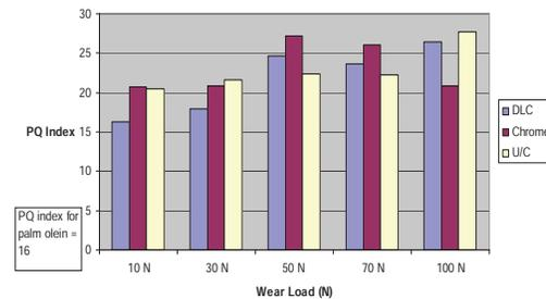
**Fig. 9 PQ index result for all used oil samples.**
