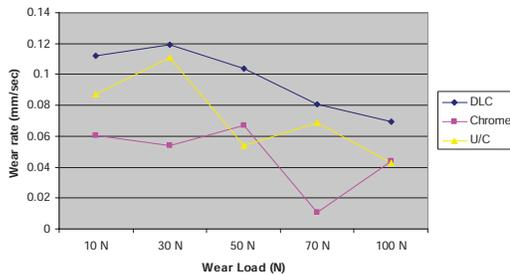
Fig 5. Wear rate (mm/sec) vs. load (N) for all samples
