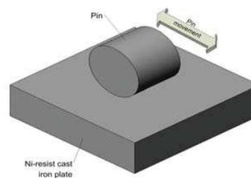
Fig. 3 Schematic diagram of the pin on disk apparatus.
