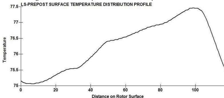
Figure 5: Mid radial temperature distribution plot for 0.5MPa
