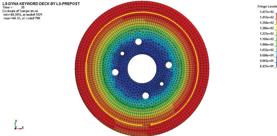
Figure 6: Surface temperature distribution profile for 1.0MPa
