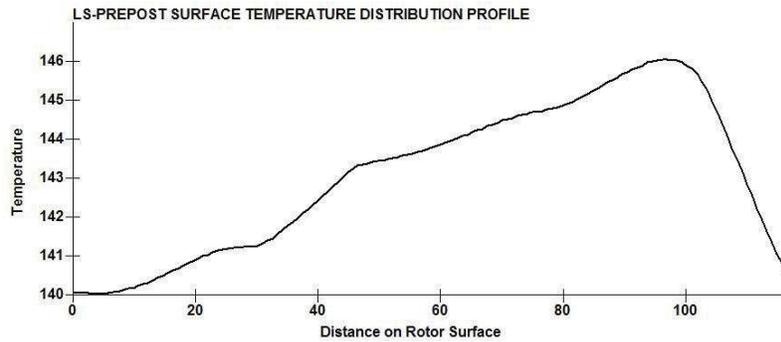
Figure 7: Mid radial temperature distribution plot for 1.0MPa
