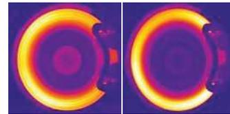
Figure 8: Thermograph analysis for average surface temperature profile for AMC and cast iron brake rotor.
