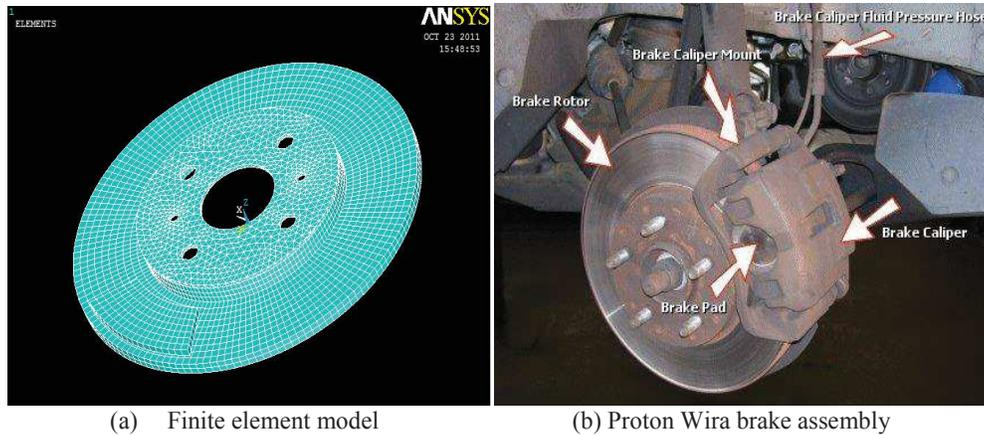
Figure 1: Brake rotor assembly
