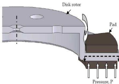
Figure 2: Thermal boundary condition
