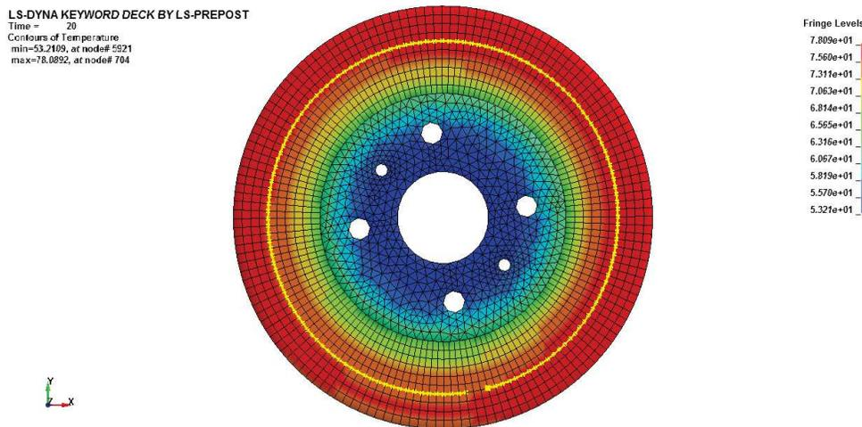
Figure 4: Surface temperature distribution profile for 0.5MPa
