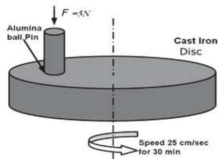
Figure 1 A schematic diagram of pin on disc wear tester under dry sliding condition.
