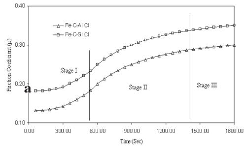
Figure 6 Friction coefficient of both conventional Fe-C-Si CI and Fe-C-Al cast iron.
