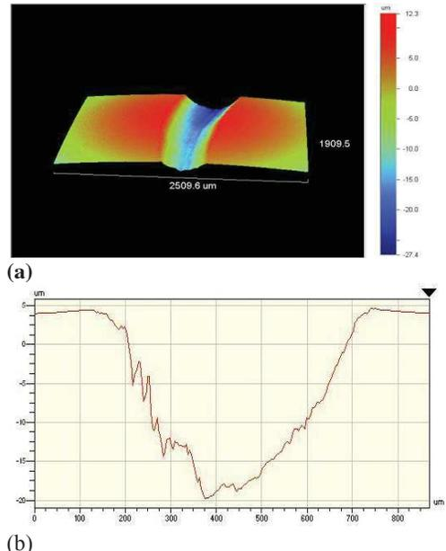
Figure 4 Wear tracks of Fe-C-Si cast iron under optical profilometer: (a) wear track profile and (b) corresponding depth of wear track.
