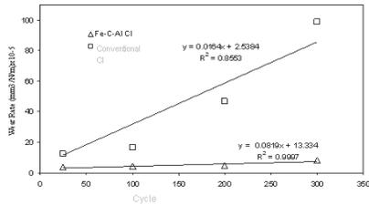
Figure 2 Wear rate of Fe-C-Al and conventional Fe-C-Si cast irons under dry sliding condition. The speed is 25 cm/s; load 5N; duration 5 min.
