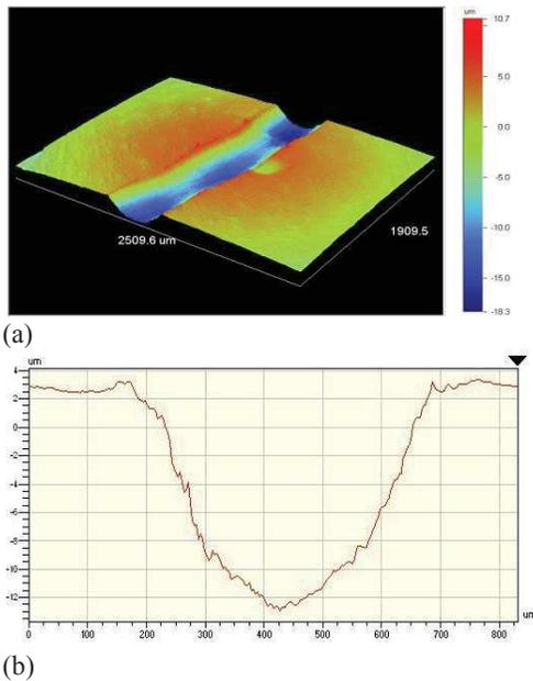
Figure 3 Wear tracks of Fe-C-Al cast iron at room temperature under optical profilometer: (a) wear track profile and (b) corresponding depth of wear track.
