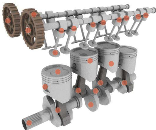
b) Four stroke inline engine
