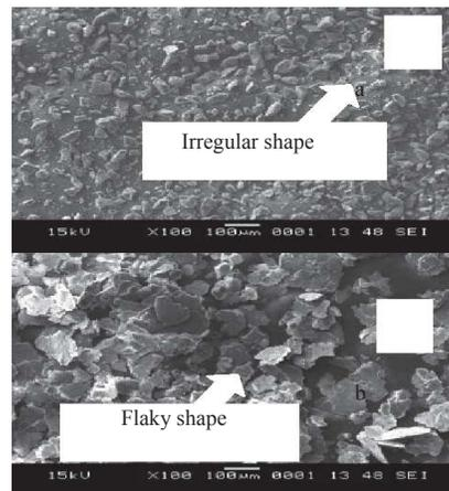
Figure 1 SEM micrograph of: (a) PSAC particles; (b) Aluminium particles
