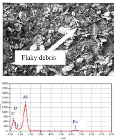
Figure 5 SEM micrograph of collected flaky debris particles of Al/20 wt. % PSAC and its EDX analysis showing C, Al, O, and Fe.
