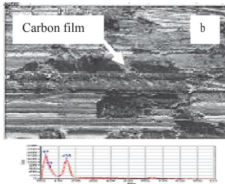
Figure 2 (a) SEM micrograph of Al/0 wt. % PSAC and its EDX showing the presence of Al and O elements. (b) SEM micrograph of Al/10 wt. % PSAC and its EDX showing the presence of carbon film on the worn surface.
