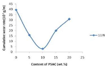
Figure 3: Cumulative wear rate versus content of PSAC at 400 m sliding distance under applied load of 11 N.
