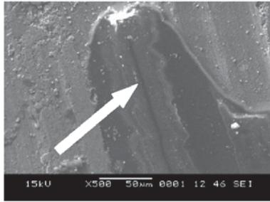
Figure 4: SEM micrographs showing the worn surface of Al/10 wt. % PSAC at applied load 11 N after 400m sliding distance indicating the black film on the worn surface with a pattern of “shear wedges” and magnified view of box is shown in figure revealing a good adhesion of black film to the worn surface
