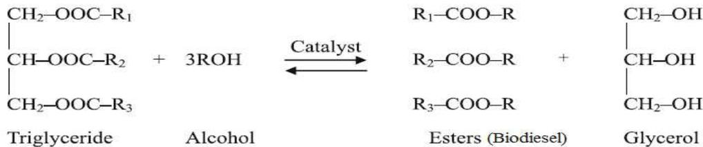
Fig. 1 Transesterification reaction of triglycerides
