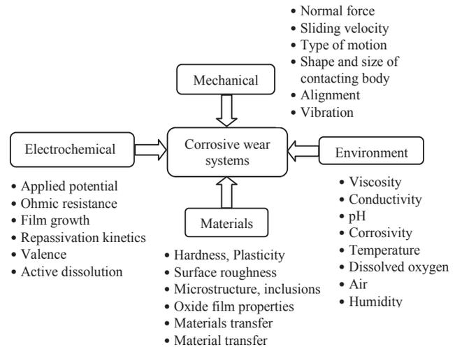
Fig. 2 Factors influencing corrosive wear
