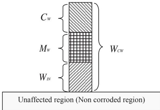
Fig 4 Model of sectioned profile of corrosive wear
