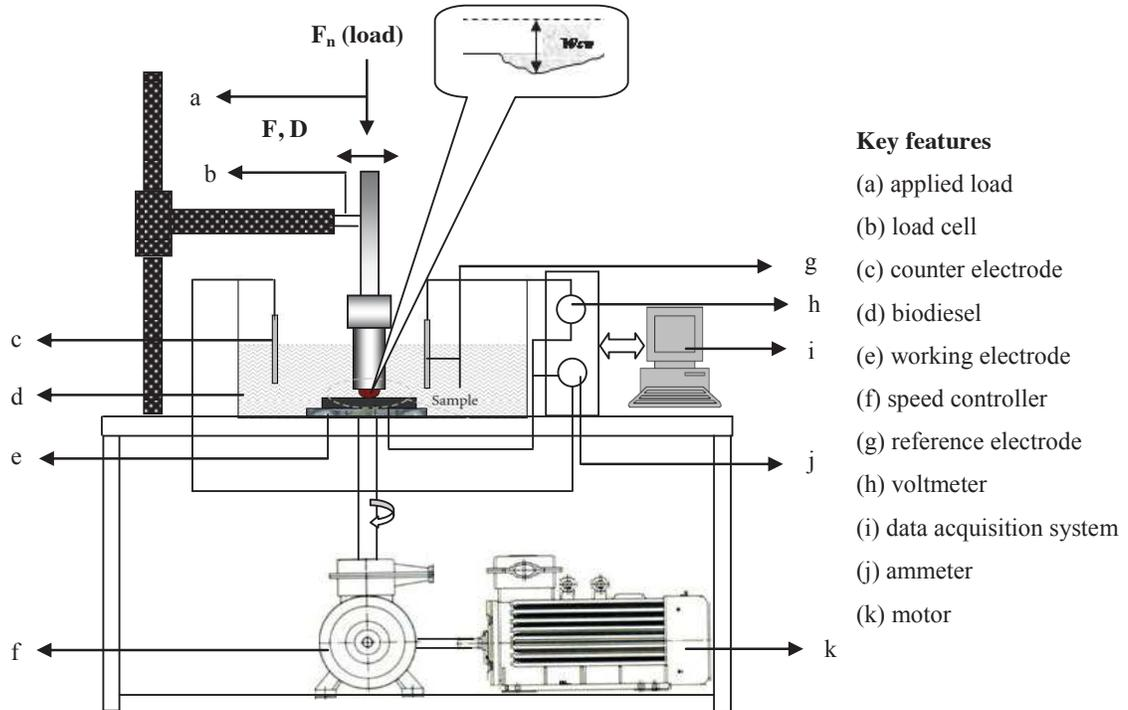
Fig 3 Proposed model for corrosive wear study of biodiesel
