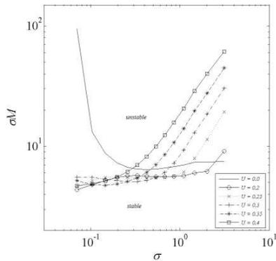
Figure 4 Stability curve for moderate to high unbalance magnitudes.
