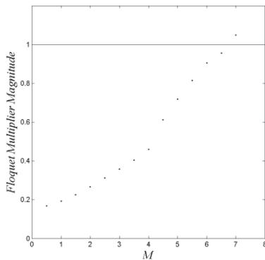
Figure 2 Magnitude of leading Floquet multiplier for  $\varepsilon = 0.3$ ,  $U = 0.2$  and the critical value of  $M$  is 6.5.
