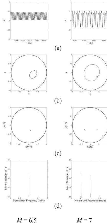
Figure 5 Rotor response for  $\varepsilon = 0.3$ ,  $U = 0.2$ ,  $M = 6.5$  (stable) and  $M = 7$  (unstable), (a) time series, (b) whirl orbit, (c) Poincaré map, (d) power spectrum.
