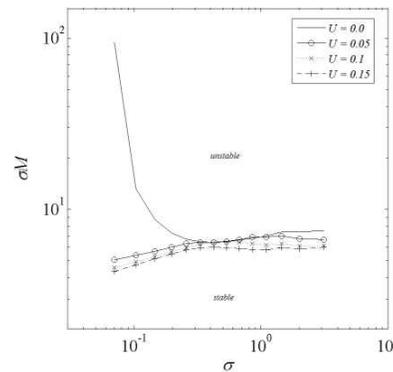
Figure 3 Stability curve for small unbalance magnitudes.
