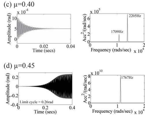
Figure 6 Time History and Power Spectral Density results for different value of friction coefficient,  $\mu$ .
