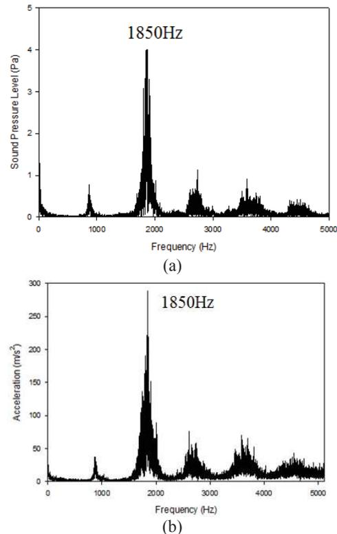
Figure 3 Fast Fourier Transform (FFT) during squealing. (a) Sound Pressure Level of squeal (b) Vibration level of leading shoe.
