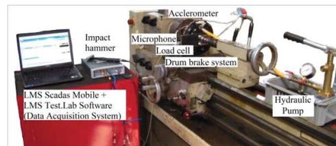
Figure 2 Experiment setup for spectrum analysis
