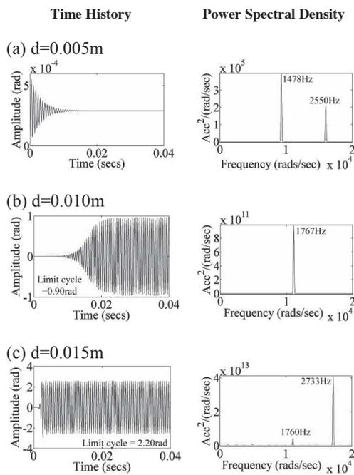
Figure 7 Time History and Power Spectral Density results for different location of centre of contact pressure at  $\mu=0.50$ .
