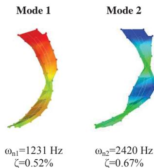
Figure 1 The first two modes of the brake shoe in free-free condition
