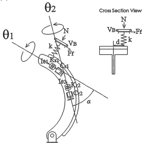
Figure 5 (a) The leading drum brake shoe;
