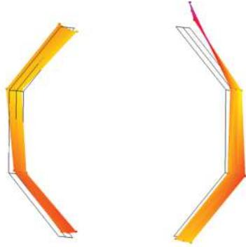
Figure 4 ODS of the trailing brake shoe during squealing at 1850Hz
